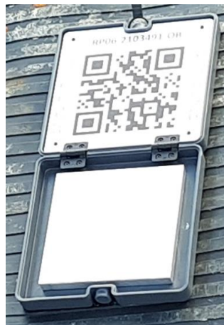
Figure 29: MicaSense sensors include a grey plastic box containing a QR code and a large white square which is the panel used to calibrate reflectance.
