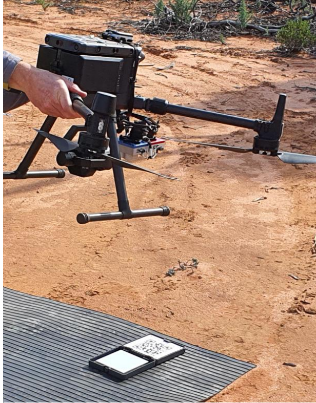
Figure 31: MicaSense panel capture: ensure there are no shadows cast on the panel or the DLS on the drone.
