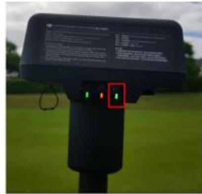
Figure 9: Power up the antenna. Press the Mode button to operate in Mode 5 – indicated by a blinking pattern of 5 times.
