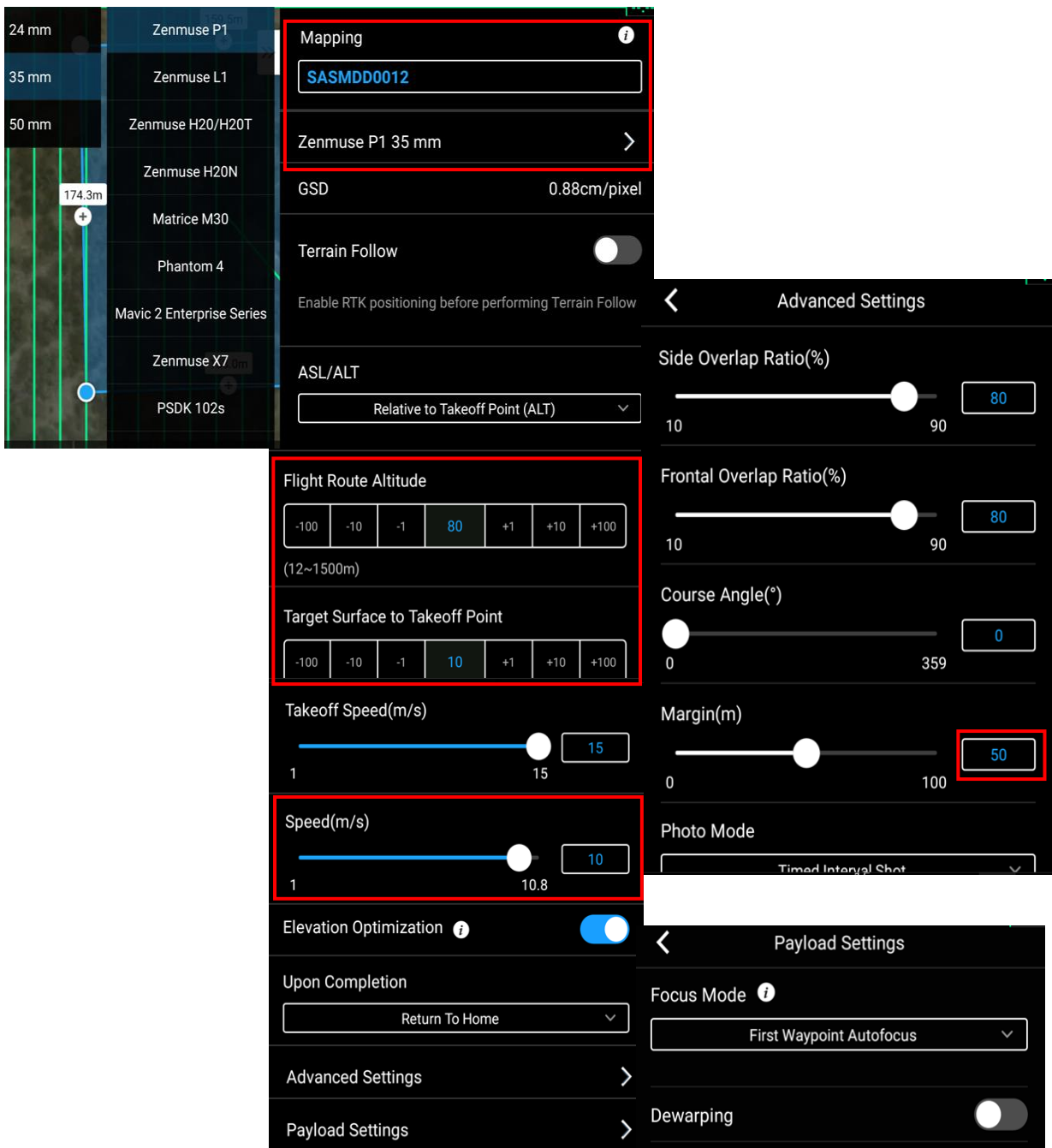
Figure 23: Mission settings: Check and update all the settings. Note that the Flight Altitude and Target Surface to Takeoff Point must be updated for densely vegetated forest sites, and in sites with a large difference in terrain to ensure adequate overlap at top of canopy/high terrain. Speed must be set to a value slightly less than the maximum possible to ensure that P1 and MicaSense trigger at similar intervals. A margin of 50 m is recommended to ensure adequate coverage on the orthomosaic.
